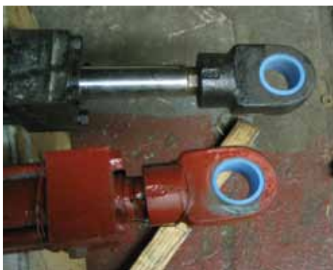
ThorPlas-Blue steering and linkage bearings installed
